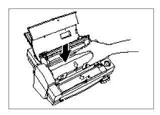
(4) Install the new film cartridge carefully.
